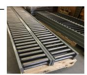
Free Standing Roller Conveyors-2" diameter, 12 gauge rollers on 3" centers, 12" overall width, with 2 heavy duty stands
