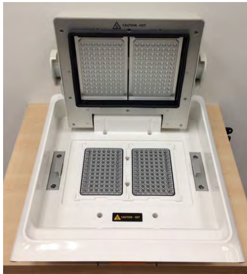
Figure 43 Location of the safety label on the ProFlex™ Dual 96-Well Sample Block
