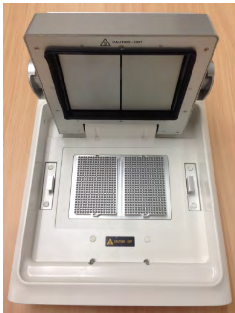
Figure 45 Location of the safety label on the ProFlex™ Dual 384-Well Sample Block
