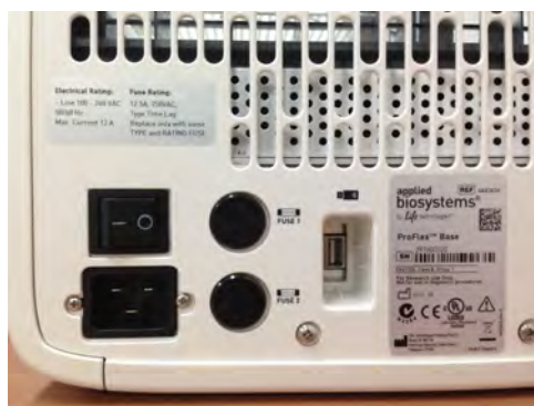
Figure 40 Location of the safety label on the rear panel of the ProFlex™ System
