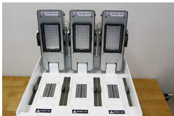
Figure 41 Location of the safety label on the ProFlex™ System 3x32-Well Sample Block
