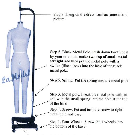
Step 2. Foot Pedal. Put the Foot Pedal on the side of the base
