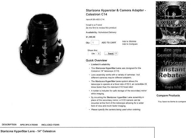
The HyperStar 14 system allows extremely fast, wide-field CCD imaging with the Celestron 14" SCT. The lens replaces the secondary mirror on Fastar-compatible 14" SCTs and turns the telescope into an f/1.9 imaging system!
